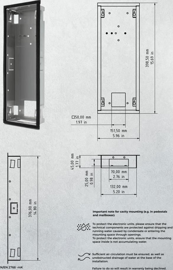
General tolerance DIN/EN 2768 -mK Wall cut-out dimension +4 mm/0.15 in
